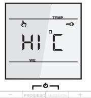
HI °C appears on the display when the surface heating is more than + 45° C.
