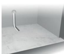
The subfloor should be even, secure, solid and with an appropriate load capacity. The surface has to be dry, clean, free of grease, dust and sharp objects. If the subfloor is uneven, it is necessary to level it, using a self-leveling floor compound before installation of the heating mat, in order to avoid air cavities underneath the heating mat. Never install the heating cable over a building expansion joint.
